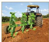
The most used soil preparation system in the world use the MOULDBOARDS PLOWS. They are the only implements that completely loosen the soil at the desired depth and simultaneously incorporate the remains from previous crops with perfection.
